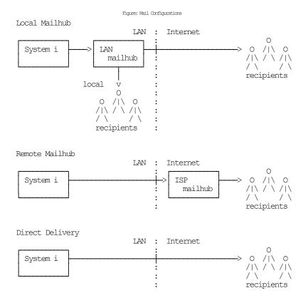
For most customers the System i is attached to a local area network that also has a mail server attached to it. Typically, the mail server runs on a PC with Exchange, Domino, SendMail, or similar mail application installed. In addition, typically, this mail server should be responsible for delivering mail, and will server as the forwarding mailhub server for the System i. If this is you situation, proceed to the Quick Start Mail Set Up - Mailhub section.
